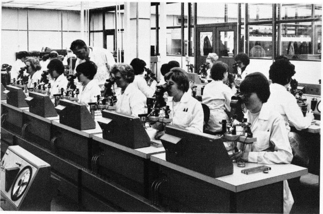
BELOW: A section of Assembly at Witham where contacts are welded. The girls are using bonding machines developed and produced by the Company. Microelectronics manufacture is now being carried out in five units at Witham. The original production unit was set up at Baddow Laboratories
